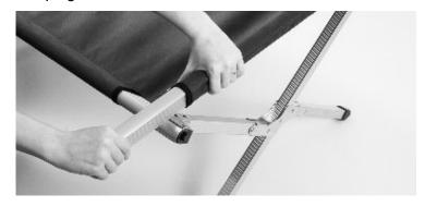
**3.** Attach one end-rail by aligning slots in this part with round tabs on side-rails and press into place.
