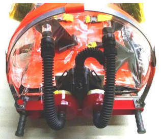
Primary filters on blower
